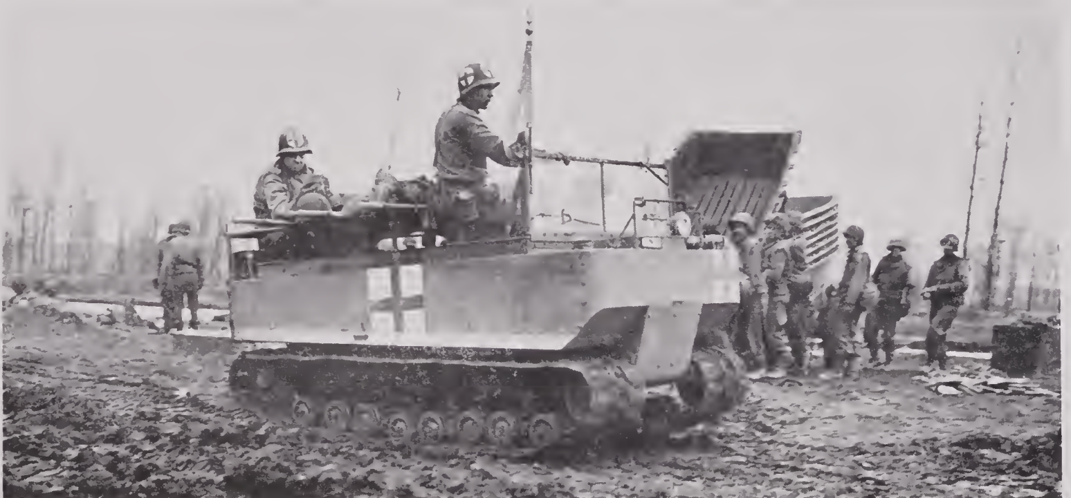
FIGURE 63. Near Roer River in Germany, a 9th Army M-29 Weasel fills its major role: evacuating casualties.
